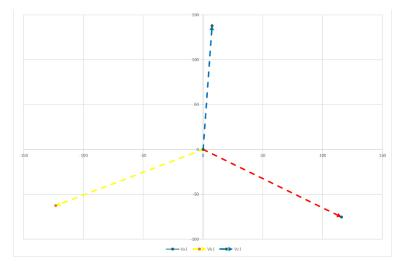
Now look at the position of phase 1 represented by the dashed red line. The entire positivesequence component has shifted in a clockwise direction. Secondly, look at the length of the dashed lines. They should be of the same length as in the previous image. This clearly shows that there is a problem.
