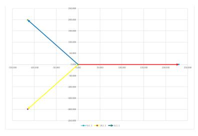
Notice that the three phases are equal in length and displaced by exactly 120-degrees. Also notice the placement of phase 1 which is represented by a red line. It is on the X-axis and towards the right-hand side of the Y-axis.
