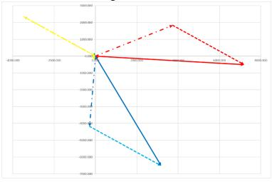
The image above shows the how the three symmetrical components that make up the voltages as recorded at 03:40:00 on September 5, 2023.
