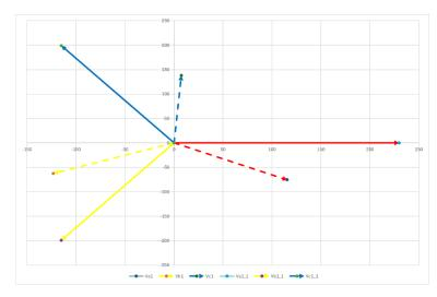
The solid-lines represent the positive-sequence voltage components of a perfectly balanced network while the dashed-lines represent unbalanced positive-sequence voltage components.
