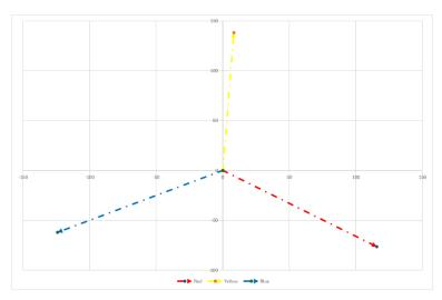
I want to point out that phase 1 represented by the red dashed line is at the same angle and magnitude as the red dashed line in the image above, the positive-sequence voltage component.
