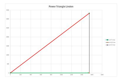
What is important and unnoticeable is that the apparent power is increased significantly due to other *inefficient powers* caused by the imbalances and there is absolutely nothing the customer can do about that, **but he is made to pay a premium for something over which he or she has no control**.
